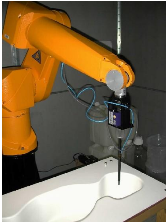
Photo courtesy U.S. General Accounting Office A probe attached to a mechanical arm is directed to take SAR measurements throughout a human-shaped mold. The mold is filled with a liquid mixture that simulates the electrical properties of human tissue.
